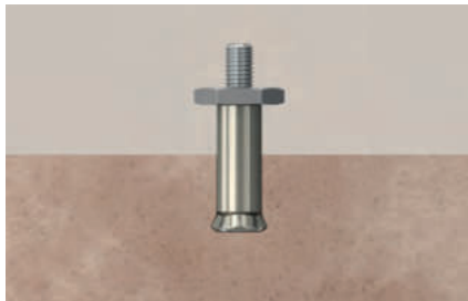
Undercut anchor in soft natural stone
