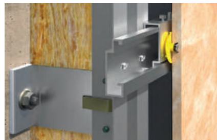
Façade cross-section with ceramic anchor
