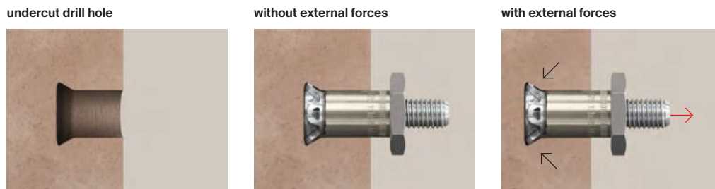
Undercut hole and behaviour of the Zykon panel anchor FZP II with and without external force
