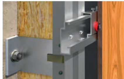
Façade cross-section with FZP II T PA
