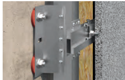
SystemOne Light in façade cross section with natural stone
