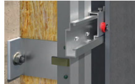
Façade cross-section with Tergo+ anchor
