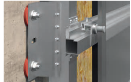
Façade cross-section with laminated composite safety glass
