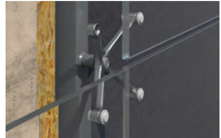
Façade cross-section with single layered glass panel
