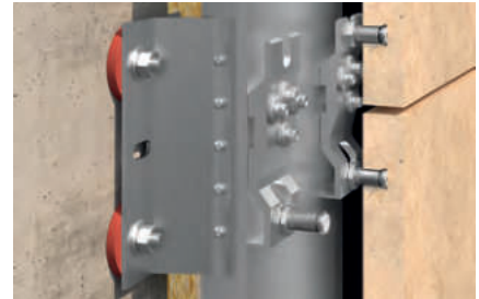
Façade cross-section with suspension anchor
